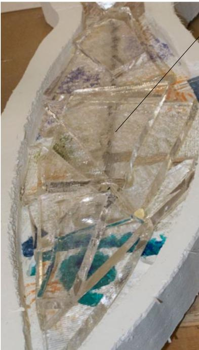
Glass in the third layer is placed well away from the edges of the mold which will cause glass to flow from the center outward.
