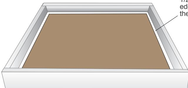
1/2 to 3/4-inch reservoir between the edge of the clay the wood frame around the perimeter form the walls of the mold.
