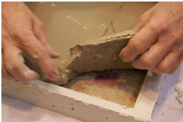
Once the plaster is set (about half an hour), Gerry removes the wood frame and turns the mold over to remove the clay.
