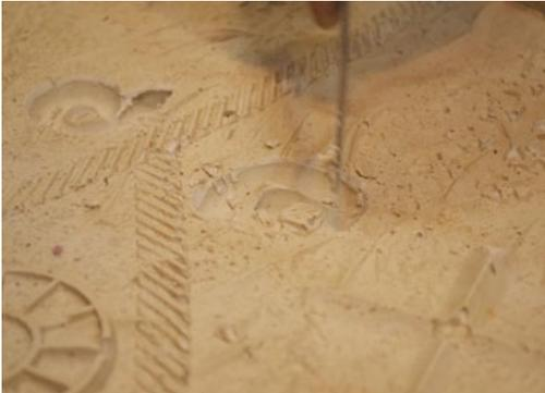
More substantial bits of clay are removed manually then the mold is rinsed quickly with water to wash away remaining residue. Gerry says that a Water Pic works well, if small. Also, a garden hose spraying through a 1/16th-inch pinhole. Note: the fresh plaster is not very hard yet; too much pressure or abrasion will erode details. Aim for a spray of water strong enough to loosen clay residue, but not abrade the mold.
