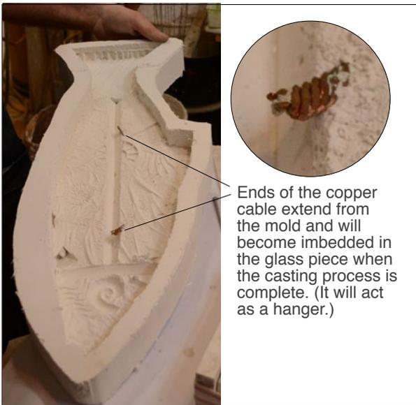
This fish-shaped mold that Gerry previously created for one of his salmon castings is dry and ready to be filled with glass. Notice that a length of sturdy copper cable extends from the plaster mold. The cable had originally been inserted in the clay version of the fish. The plaster captured it and now only the ends are showing, for the glass to bond to. During the casting process, the ends of the cable will become firmly imbedded into the glass and will be strong enough to hang the heavy fish.
