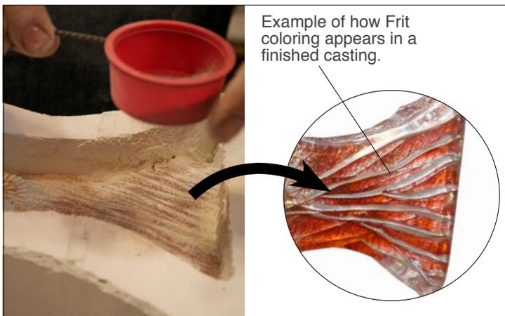
Gerry adds color, texture, and interest into design areas using different materials. Here, he sifts fine grade System 96® glass Frit into the tail section of the fish mold. Remember the area closest to the mold will be the surface of the finished glass piece, so these color accents will show well.
