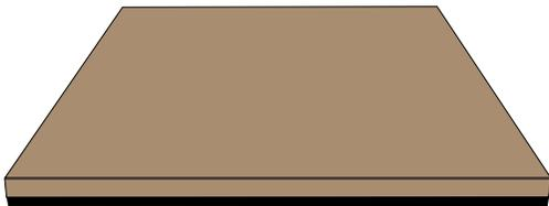
A slab of clay is rolled flat (about 3/4-inch thick). Gerry lays it on top of a rubber mat to give additional height to the mold walls (insuring that glass will not overflow). Additional clay thickness, or a 1/2-inch foam board from a hardware store can be used for the same heightening effect.
