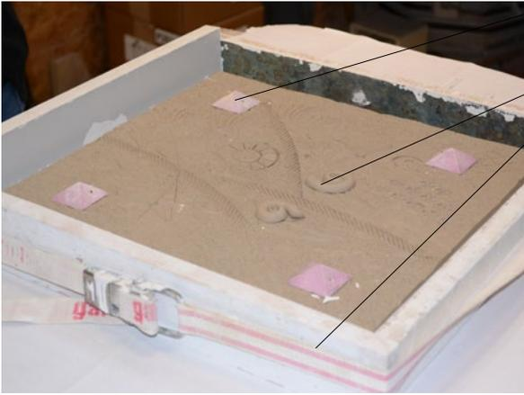
Gerry has created pyramid shapes that are made out of foam-board. A small finishing nail is used to “pin” them into the clay so they don’t float away in the wet plaster when it’s poured in.
