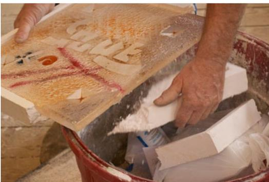
A plaster mold such as this is used only once. After the casting process, the mold has become soft, breaking away easily from the glass piece, and is discarded. Gerry explains that, while there are reusable mold mixes available, they require a mold release agent, which results in a corresponding loss of detail. Also, design undercuts are not possible as the glass will "lock" into the mold. The artist must choose the best materials for the artwork being created.
