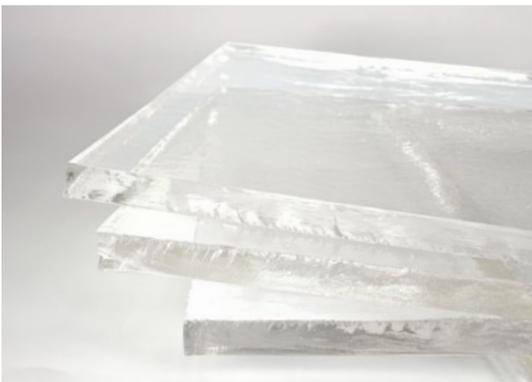
After Gerry finishes the color detail work, he fills the rest of the mold with thick slabs of System 96® **Crystal Clear Casting Plates**, carefully sized to fit into the mold and create the appropriate glass volume needed. According to Gerry, Casting Plates are nearly “bullet proof” for devit.
